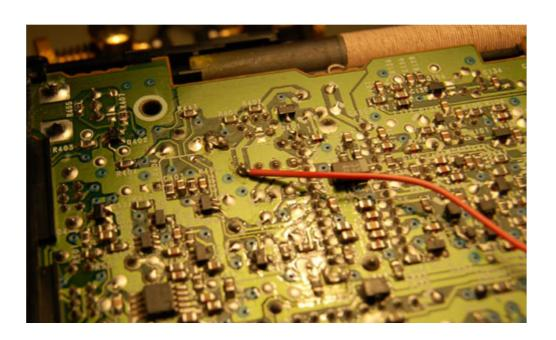
For the connection use a shielded wire and connect the shield to ground next to the signal. The other end of the wire can be connected to the line out after removing the capacitors C421 and C 423
